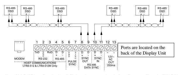
Notes: Up to 30 RS-485 Data Sync Devices (DSDs) can be connected to the Data Sync port. Since the SYNC IN port can send as well as receive, 30 extra devices can be connected. If more than 60 DSDs are to be connected, another Master Clock will have to be used as a "Booster".
